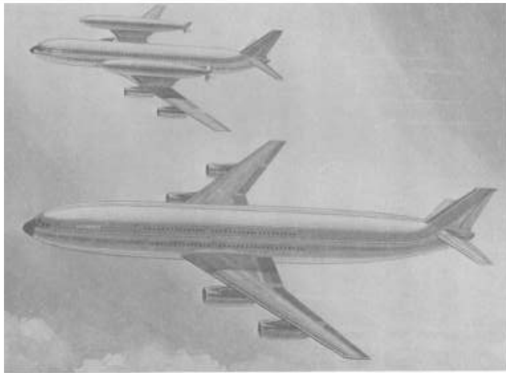
Fig. 8. Alternative design of H 2 turbojet passenger aircraft.
